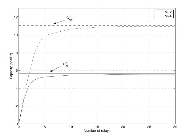
Capacity vs. number of relays for the AF relay network
